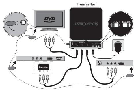
Fig. Connection example for Transmitter
